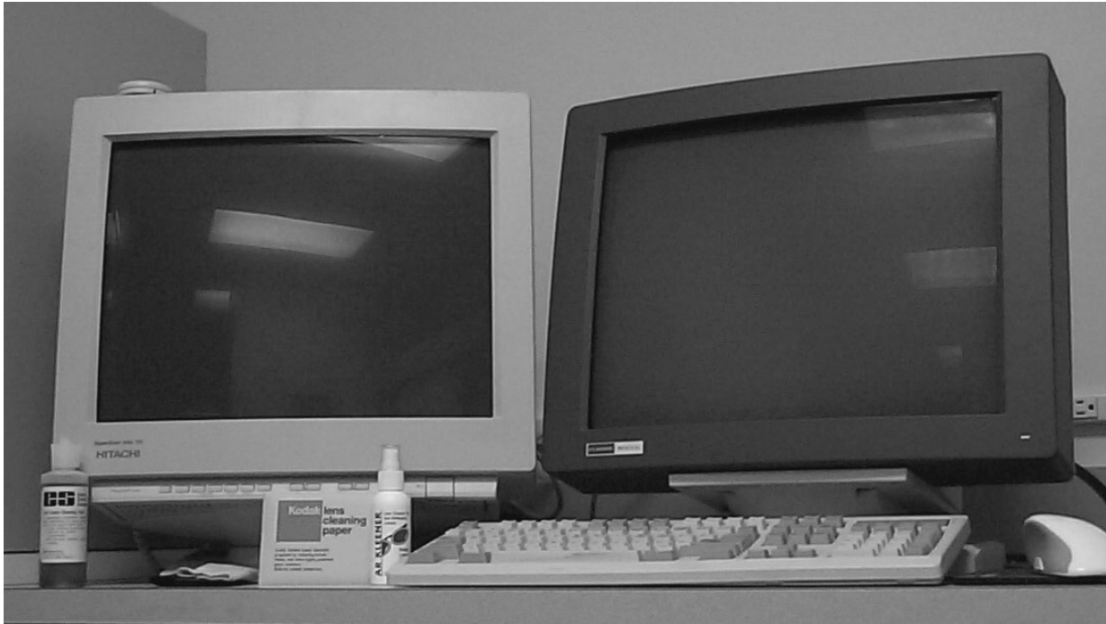
Fig. 41: Diffuse and specular reflections are illustrated for a color (left) and a monochrome (right) display device with the power off. Reduced diffuse reflections are seen in the color display device due to the black matrix emissive structure. Reduced specular reflections are seen in the monochrome display device due to an improved anti-reflective coating.
